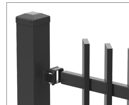
4x FB3825-2H Brackets per panel, 2x TEK121420 Screws per bracket
