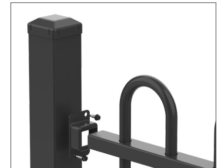
4x FB3825-2H Brackets per panel, 2x TEK121420 Screws per bracket
